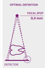
Sharp images at all times RXDC - HyperSphere technology provides your surgery with optimum X-ray quality whatever the type of sensor connected. Now even more powerful, with 70 kV and 8 mA, even more flexible and suitable for all commercially available sensors. The constant potential head tube, associated with the smallest intraoral imaging focal spot available (0.4 mm), ensures the best images whatever your diagnostic needs.
